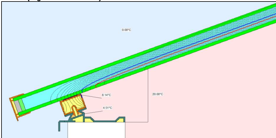
Simulation model (detail) with insulating glass unit (isothermal lines at 0°C externally / 20°C internally)
