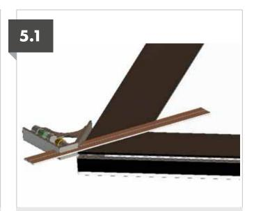
Ensuring glazing unit is positioned with bottom/laminate pane facing upward, take each section of FRL5402BK-Structural Glazing Tape remove lower section of adhesive backing film and position on corresponding edge of the glazing unit taking care to all edges and mitred corners are in-line and match.
