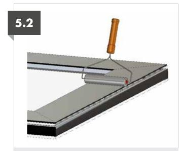
Use hand roller to ensure FRL5402BK-Structural Glazing Tape is fully adhered to glazing unit and all air pockets between contact surfaces are disbursed.
