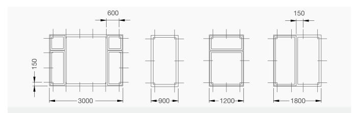
If fixing cleats is the chosen method of installation they should be attached to the outer frame starting at 150mm from the corner and thereafter at a maximum of 600mm centres. The cleats should be screwed into the mainframe in the central reinforcing chamber.
